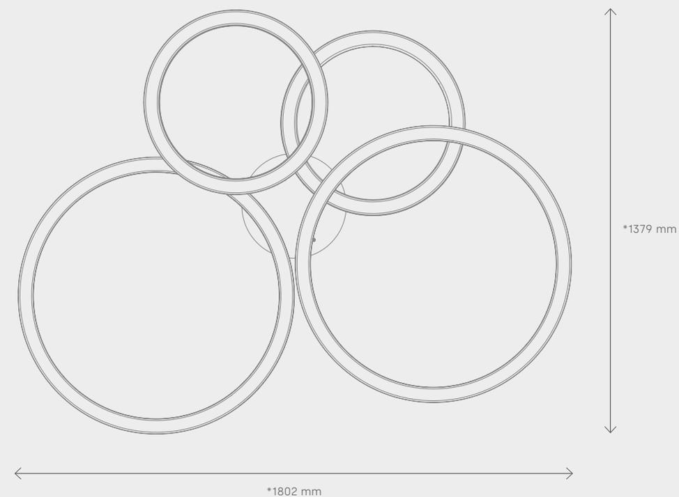
\*The figure shows an example of dimensioning, which changes depending on the individual system of circles.
