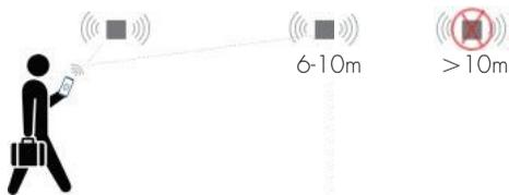
The smart device with the App installed will have a typical range of 10m, but varies from device to device. During commissioning, the installer will need to be in range of the devices when searching for devices to add to the network.
