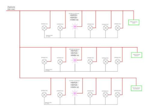
The sensors are powered by a 3x2.5 mm2 cable and the DALI bus is connected to the lamps within a given zone as shown in the diagram.
